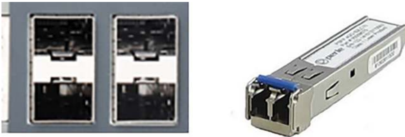
FIGURE 6.2 Small form-factor pluggable interfaces
